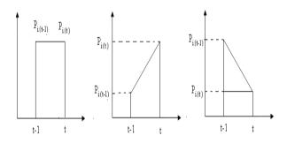
Fig. 2. Ramp rate limits of generating units
