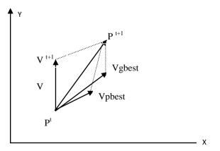
Fig. 3. Concept of modification of a searching point by PSO
